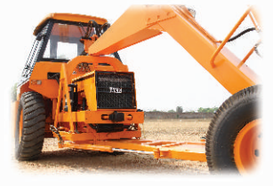
3 STEERING CYLINDERS 880 mm stroke cylinders ensure proper steering even in loose, sandy & rocky terrains.
