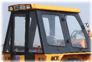
1 ROPS CABIN Wide view ROPS cabin for better visibility.
