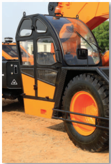
7 CABIN Front mounted, ergonomically designed Cabin for better visibility and driveability.
