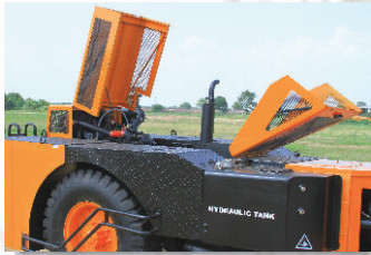
4 EASY MAINTENANCE The engine is easily accessible for daily maintenance checks including battery, air filter, oil level dipstick and cooling system.
