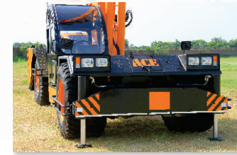
9 OUT TRIGGERS Front outriggers are provided as standard fitment for added safety during high lift operations.
