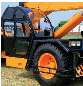
ACE FX250 Model Crane fitted with 3 part slotted boom (11.6 Mtrs. height)
