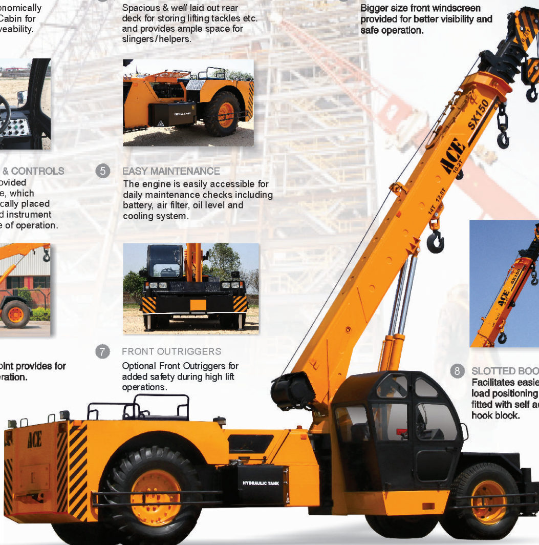
ACE SX150 Model Crane fitted with 4 part slotted boom (15.4 Mtrs. height) (4th part power extended)
